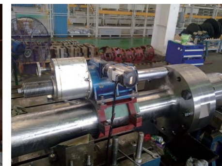
现场铰配 Field Reaming & Fitting
